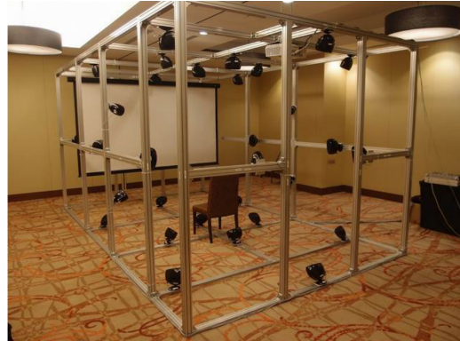
Figure 5: A photograph of the demo system. The 32-channel loudspeaker array is distributed over a metal frame housing the screen and listening space. The system is controlled by two computers, one for video presentation and one for sound rendering.
