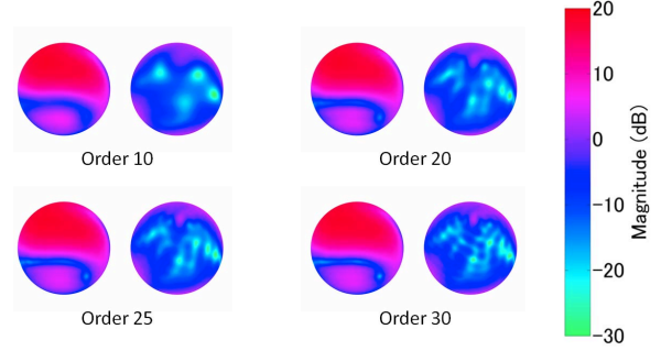
Figure 3. Reconstruction of HRTF data from a finite number of spherical harmonic expansion coefficients. The original data corresponds to 21,162 directions and a frequency of 7.4 kHz. The order 10 reconstruction uses 121 coefficients, at order 20 it comprises 441 coefficients, for order 25 this rises to 676 coefficients, and at order 30 a total of 961 coefficients are used.
